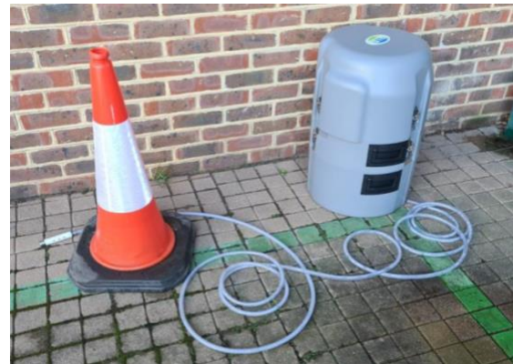
Samples were collected using manual-sampling and using Hach Autosampler, shown here
