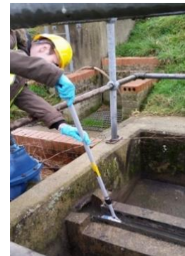
Wastewater collected using manual-sampling method
